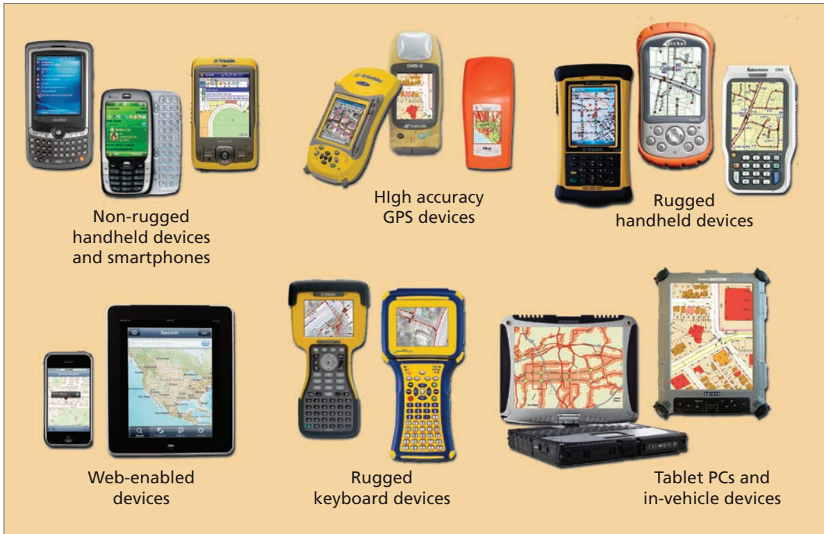
Figure 7.10 Many information products will have a mobile technology component for gathering, recording, editing, or serving data on mobile devices. Maps courtesy of City of Redlands, San Diego Metropolitan Transit System and Transportation Management & Design, Inc., and Cobb County Water System.
